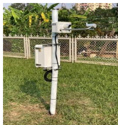
Figure 4. Disdrometer installed at Ha Dong station.
